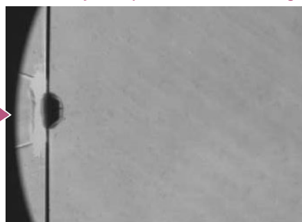
2) Instant the projectile penetrates through the aluminum plate. A small explosion can be seen.
