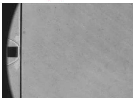
1) Left-side projectile is flying at 10 times the speed of sound. Instant before impact with the first aluminum plate.
